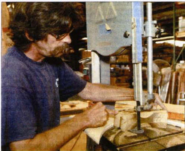
Craftsman Donald Klink manufactures custom handrail parts at Bast.
